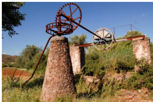
Fig. 85 - Noria with a long axle
