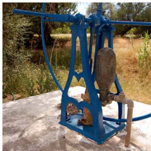
Fig. 80 - Wheel with air chamber
