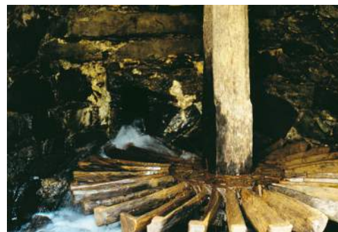
Fig. 63 - Pela" and the wood caster feather blades
